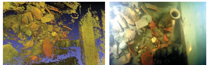
Figure 7 To the right, one of 253 photographs made on Arles-Rhône XII wreck, and in to the left the corresponding 3D points cloud.
