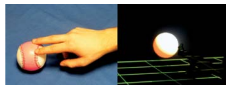
(c) Index and middle fingers both touch an object to delete it.
